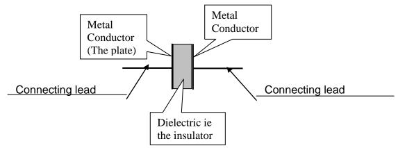
The symbol is really how the capacitor is basically constructed.
