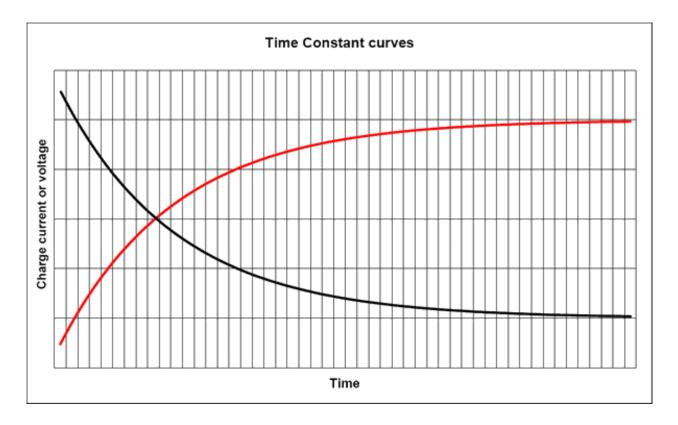
Now it takes **5 Time Constants** for the capacitor to be fully charged. (or discharged)
