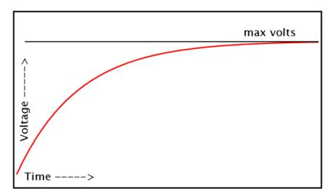
This is because the effective resistance of the capacitor *increases* as it charges up to full.
