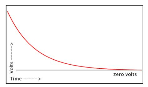
This is because as the capacitor charges up, the amount of current flowing through the resistor starts off high, but rapidly *decreases* with time, and eventually there is no measurable voltage drop across the 'series R', because once the cap is charged up, the current flow through the capacitor (& the series R) ceases.
